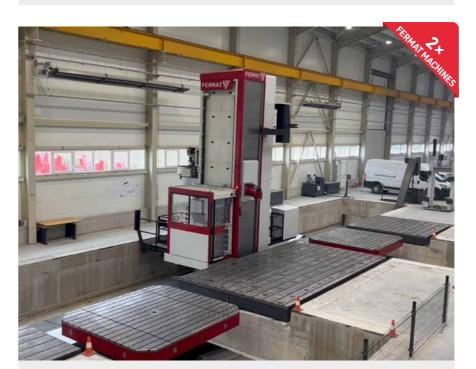
WRF Mill CNC Verarbeiten Pausits Kft. | HUNGARY Parameters:  $X = 24\,000$  mm / 945 in,  $Y = 5\,000$  mm / 197 in,  $Z = 1\,550$  mm / 61 in,  $V = 2\,400$  mm / 95 in, Rotary Table  $3\,000$  x  $3\,500$  mm / 118 x 138 in
